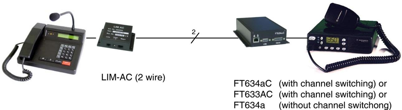
Parallel operation of multiple operator devices --> LIM AC requires notch filter option for pilot tone
